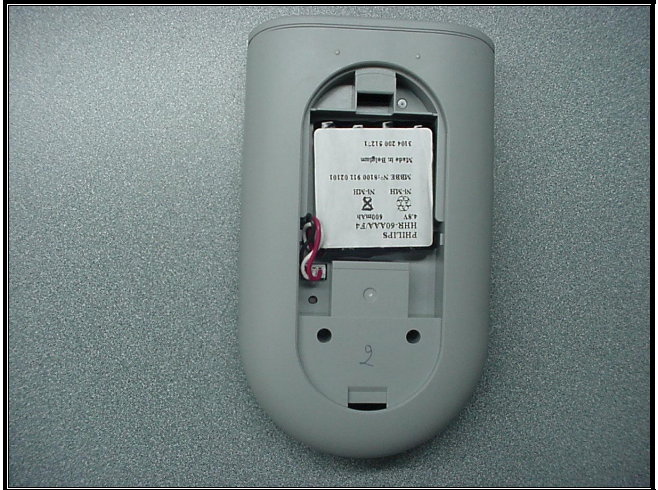
PHOTOGRAPH 17: REAR VIEW OF TOUCH SCREEN REMOTE CONTROL WITH BATTERY COVER REMOVED
