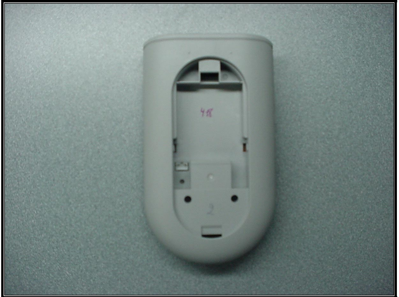
PHOTOGRAPH 18: REAR VIEW OF TOUCH SCREEN REMOTE CONTROL WITH BATTERY REMOVED
