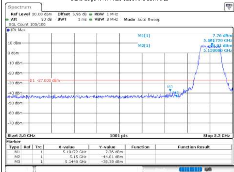
Band Edge NVNT n20 5240MHz High Ant2
