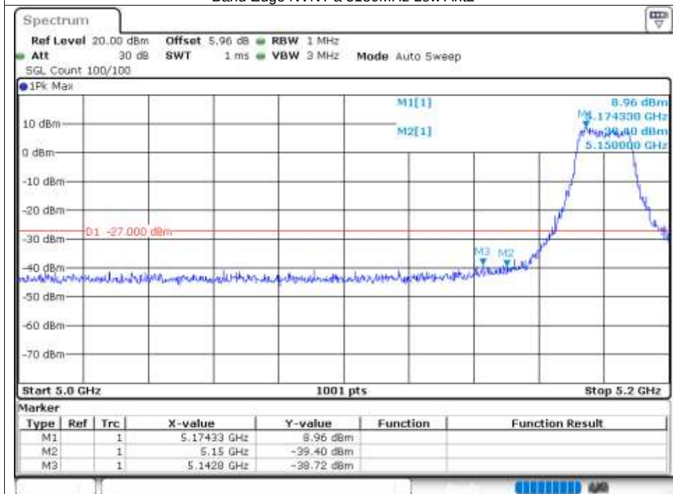
Band Edge NVNT a 5240MHz High Ant2
