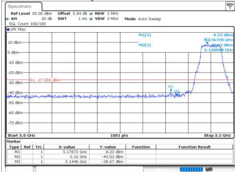
Band Edge NVNT n20 5240MHz High Ant1
