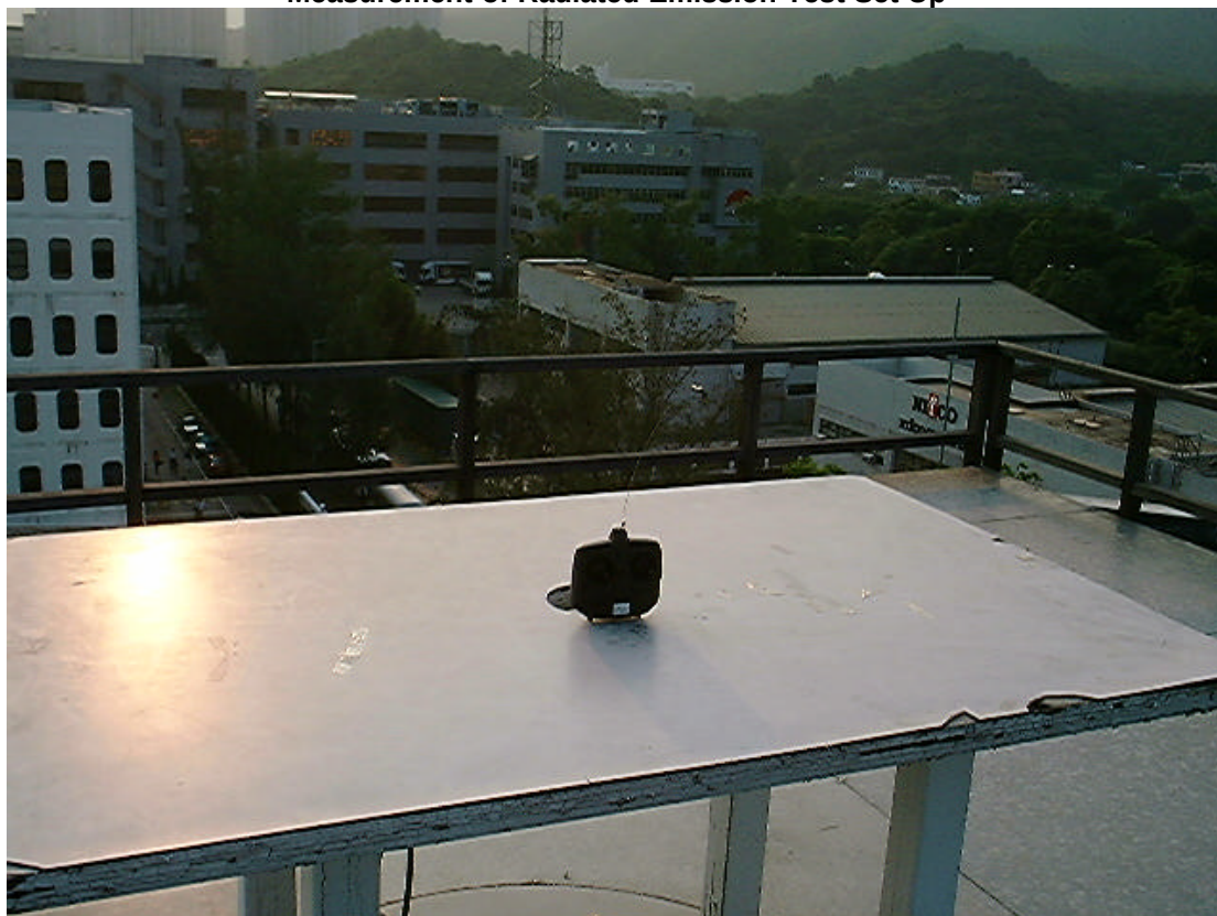
Measurement of Radiated Emission Test Set Up
