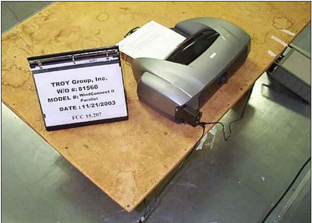
Mains Conducted Emissions - Back View Parallel
