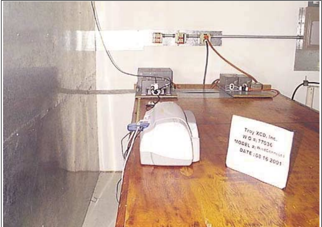
Mains Conducted Emissions - Back View (Brea Setup)
