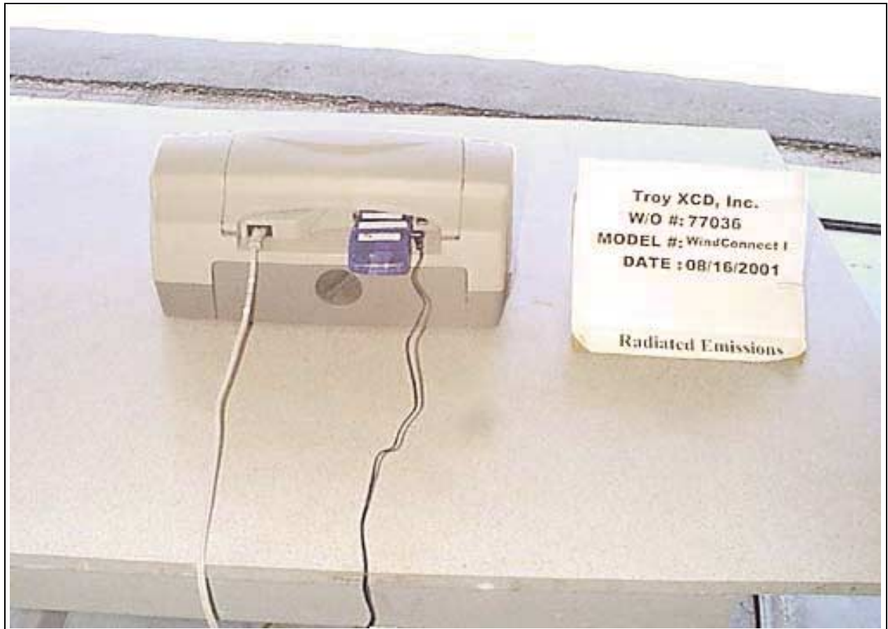
Radiated Emissions - Back View (Brea Setup)
