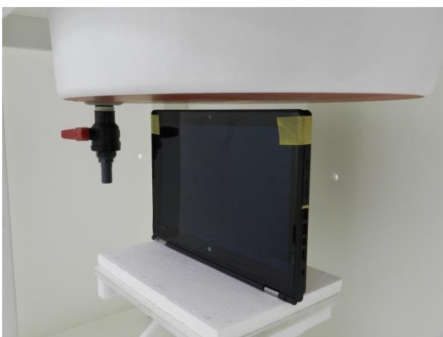
Edge1, Test Separation 20 mm
