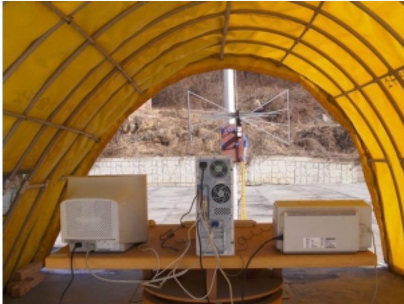
Photograph 1 : Setup for radiated Emissions
