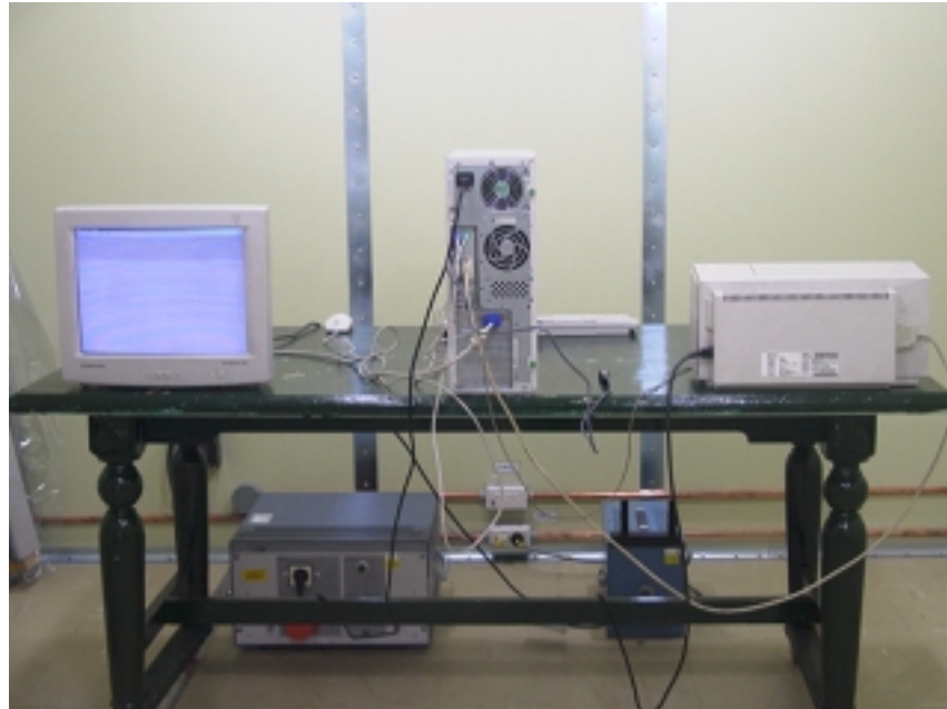
Photograph 2 : Setup for Conducted Emissions
