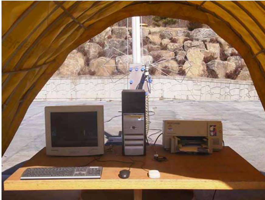
Photograph 1 : Setup for radiated Emissions
