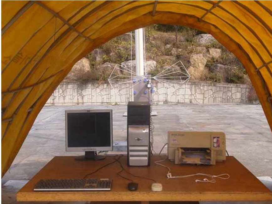
Photograph 1 : Setup for radiated Emissions
