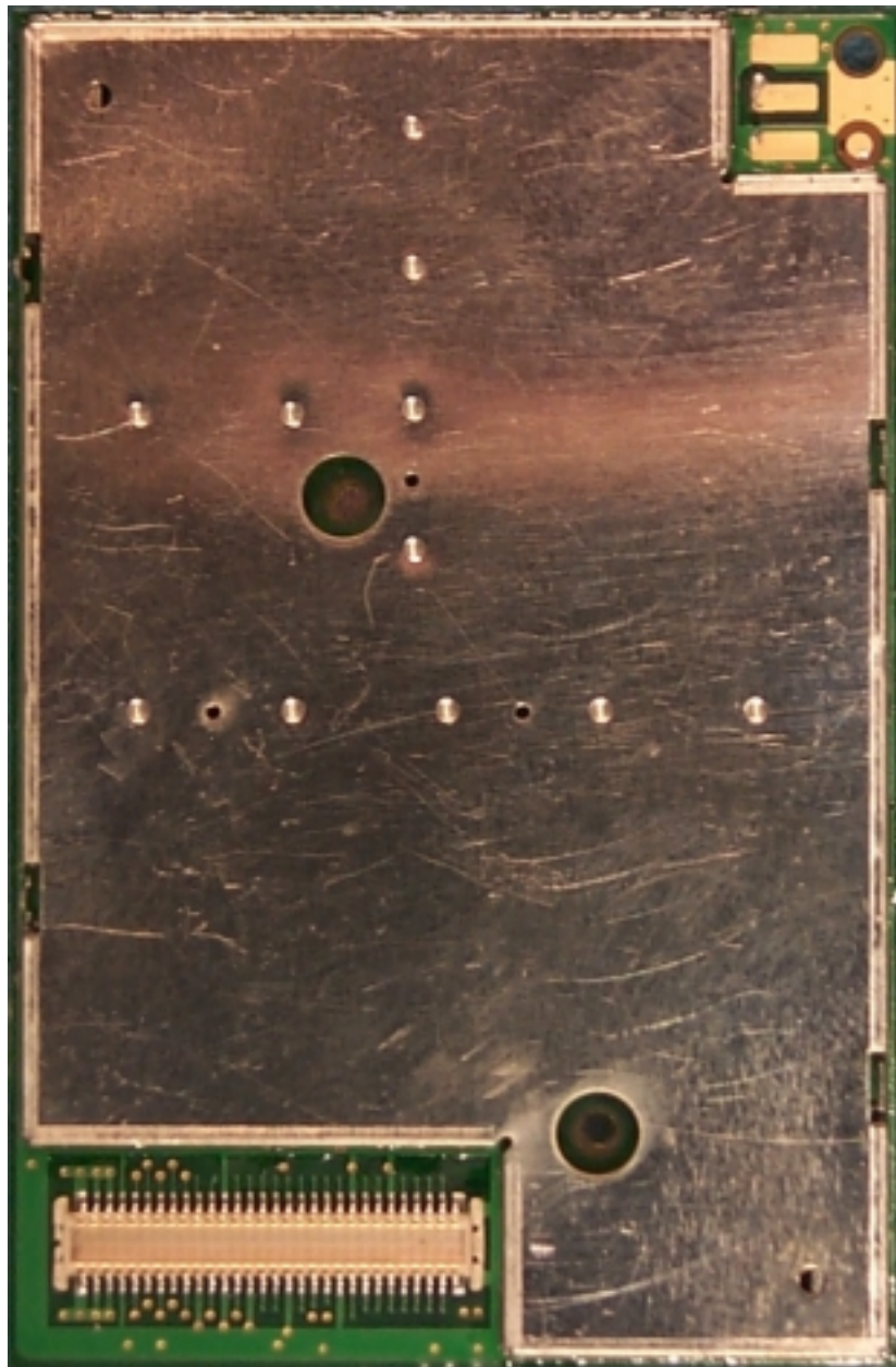
Photo 4. Bottom of Core Engine (shield in place).
