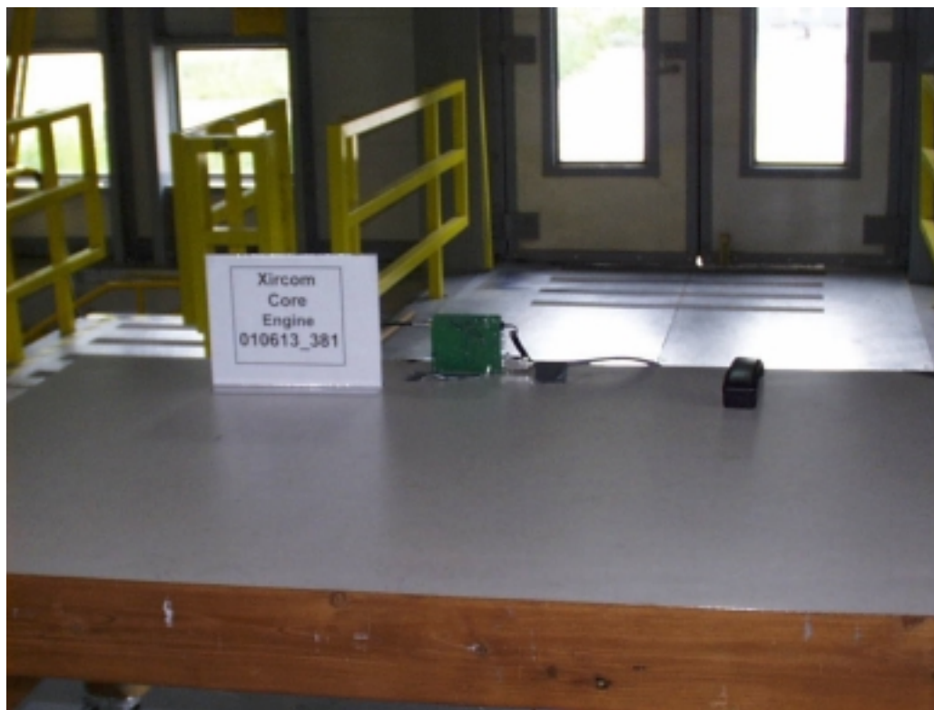
Figure E14.2. Radiated Emissions set-up at Criterion Technologies.
