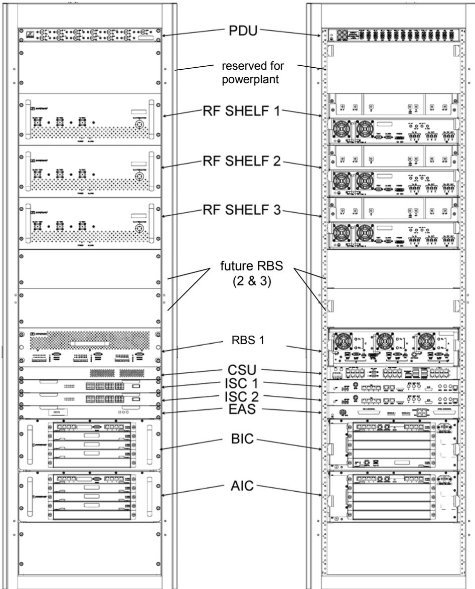
Figure 2 MC-Series System 3-sector configuration
