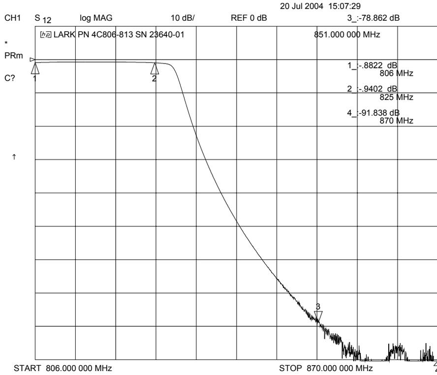
**Figure 44** Receive filter frequency response
