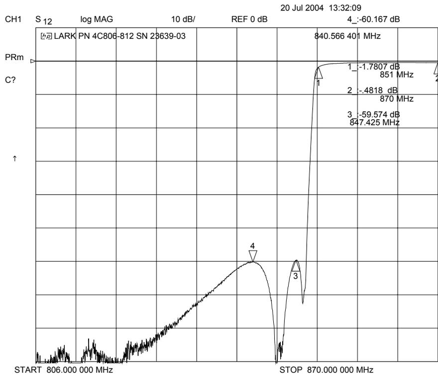
**Figure 43** Transmit filter frequency response
