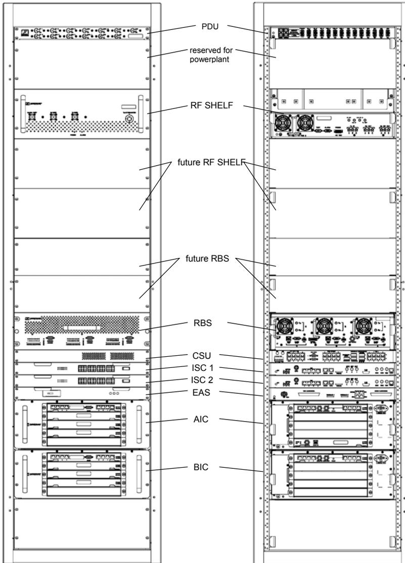
Figure 42 MC-Series System Omni Configuration
