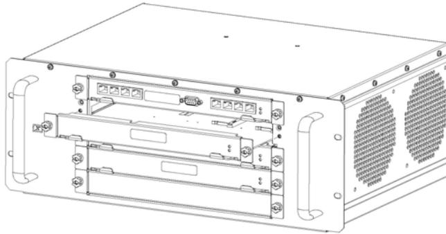
**Figure 35** Replacing the BPC in the BIC or the BPC+SPAM in the AIC.
