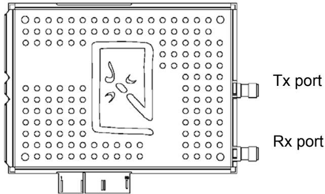
**Figure 19** iDEN 2-port RadioBlade transceiver
