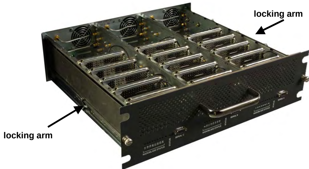
Figure 71 RF Shelf Showing Side-Rail Locking Arm Locations
