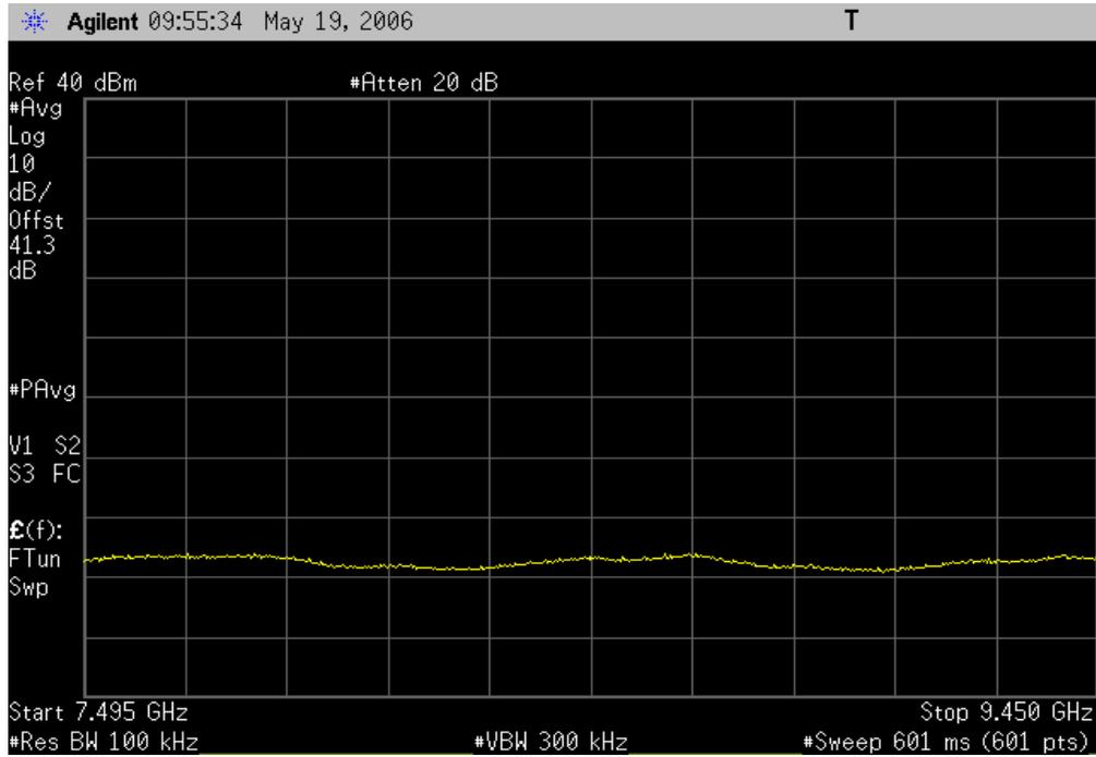
**9 Channel Intermods, In Band**      **Result:** Pass      **Value:** -22.4 dBm      **Limit:** ≤ -13 dBm
