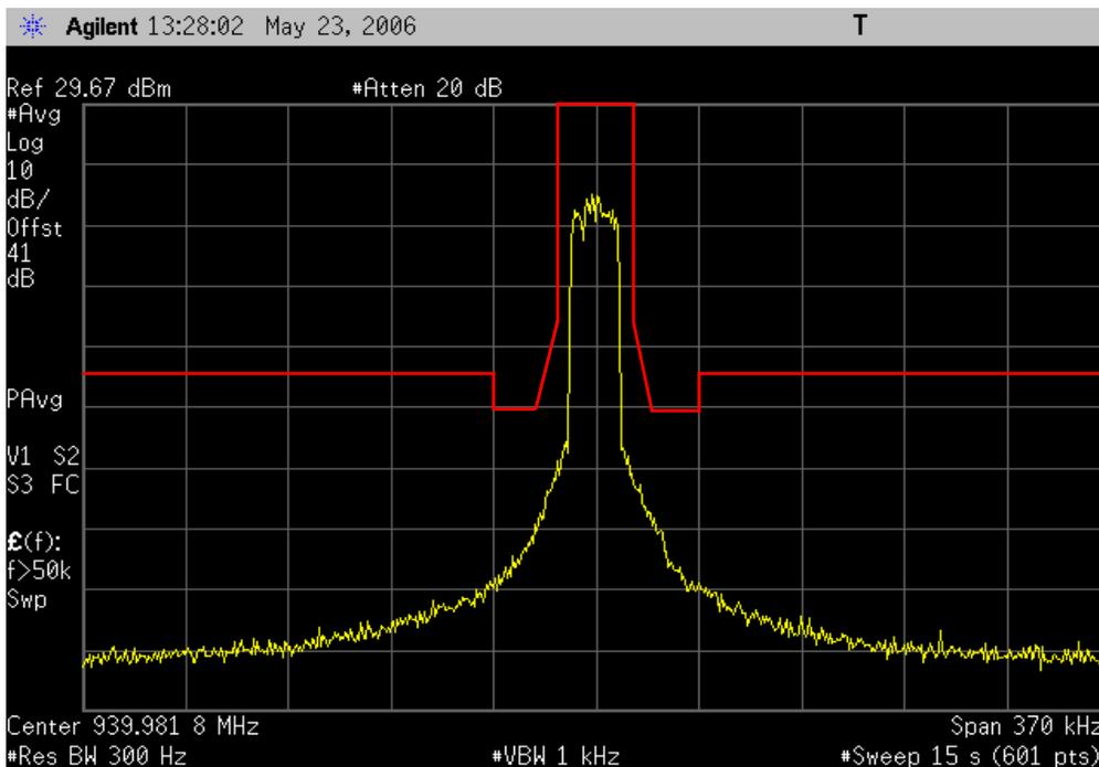
**Result:** Pass      **High Channel, Mid Power, < 37.5 kHz Fc**      **Value:** N/A      **Limit:** See Table
