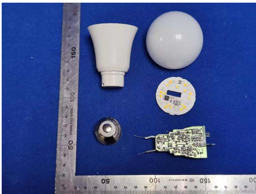
FIGURE 3 DIRECT CONNECT FULL COLOR A19 (M/N: CLEDA199CD1) COVER REMOVED
