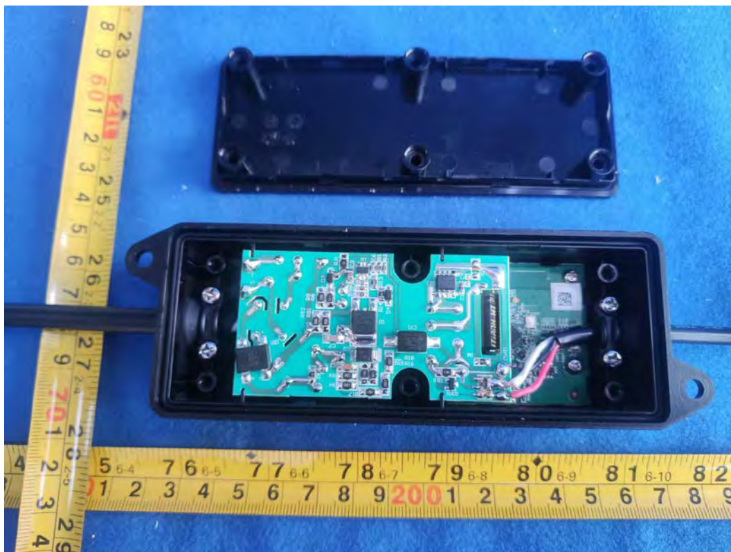
FIGURE 10 CYNCR DYNAMIC EFFECTS SMART CAFÉ LIGHTS (M/N: CCF48CDOD/ENS) CONTROL COVER REMOVE
