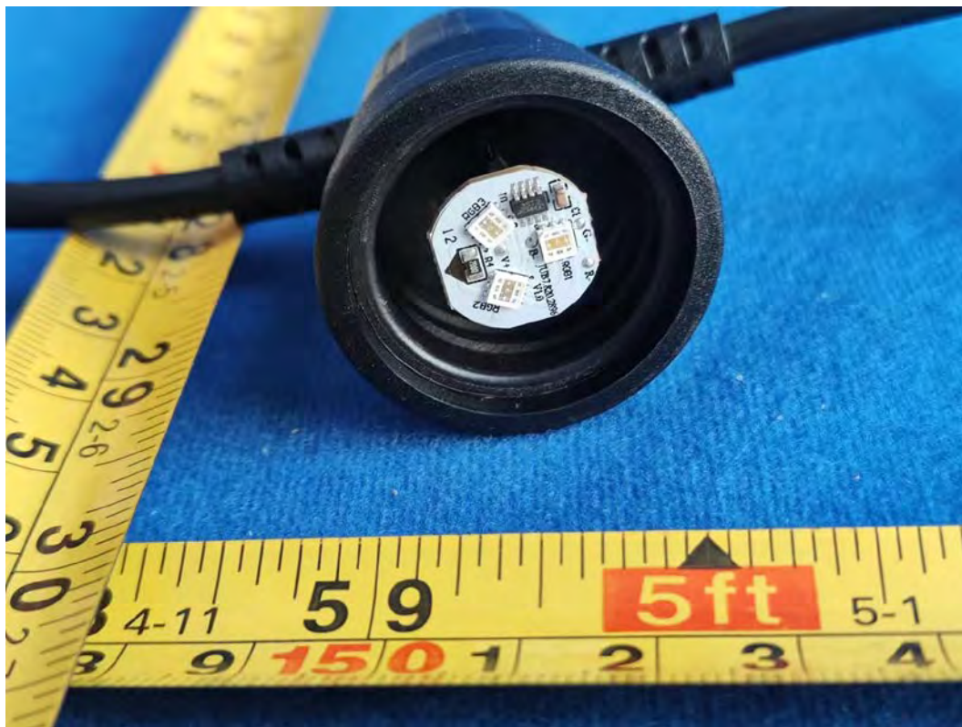
FIGURE 9 CYNCR DYNAMIC EFFECTS SMART CAFÉ LIGHTS (M/N: CCF48CDOD/ENS) BULB COVER REMOVE
