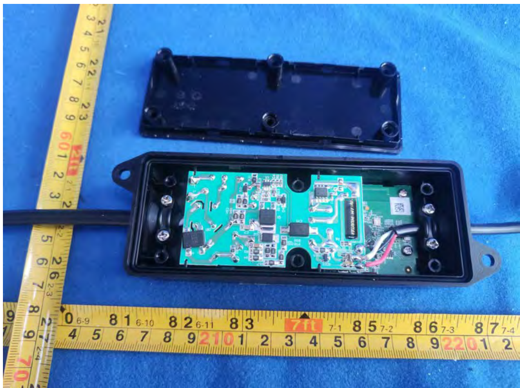
FIGURE 55 CYNIC DYNAMIC EFFECTS SMART CAFÉ LIGHTS (M/N: CCF72CDOD/ENS) CONTROL COVER REMOVE
