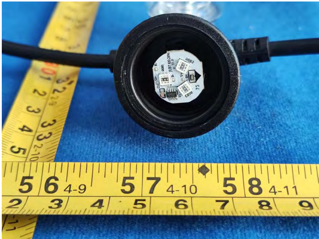
FIGURE 24 CYNC DYNAMIC EFFECTS SMART CAFÉ LIGHTS (M/N: CCF24CDOD/ENS) BULB COVER REMOVE
