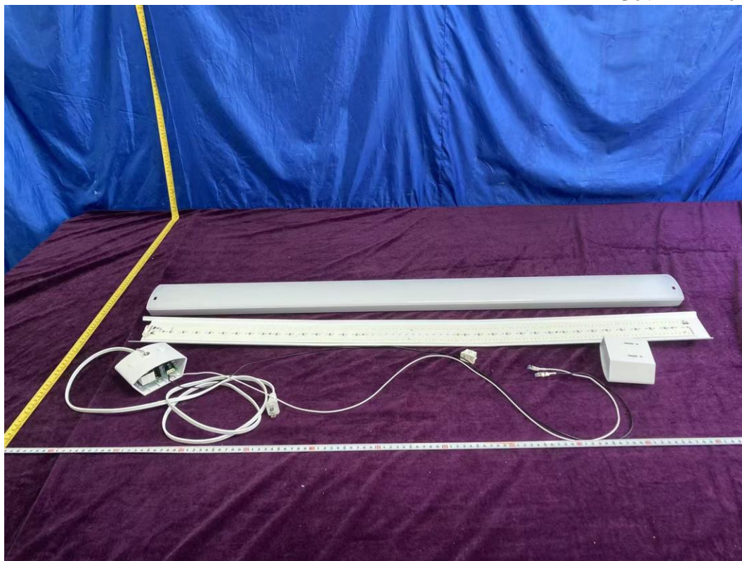
FIGURE 7 CYNC SHOPLIGHT (M/N: CFIXSHP46CDMAT) COVER REMOVED
