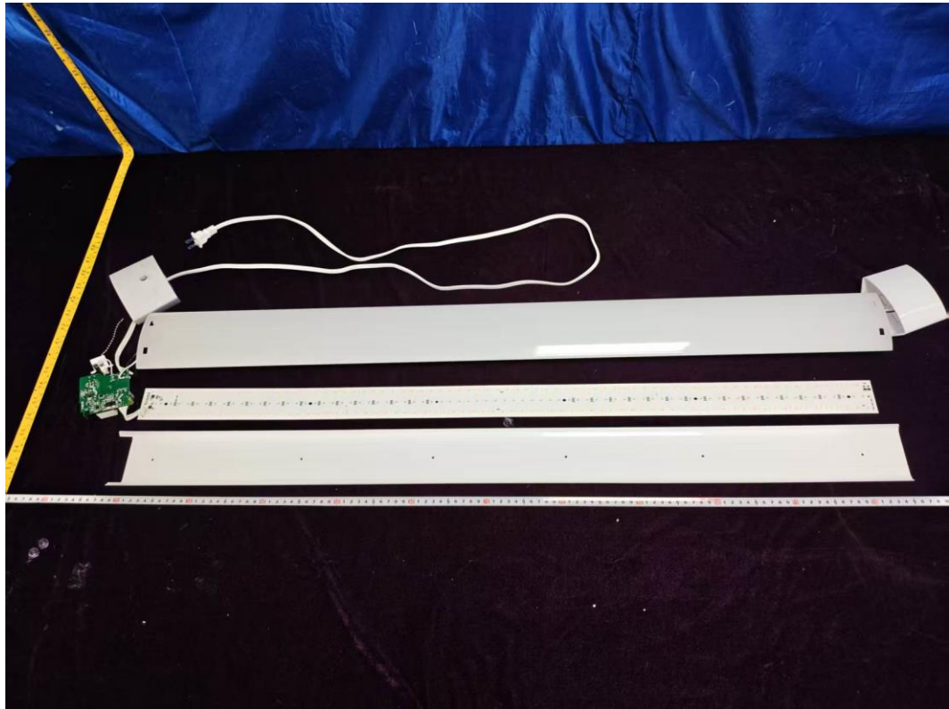
FIGURE 7 CYNC SHOPLIGHT (M/N: CFIXSHP46CDMAT) COVER REMOVED
