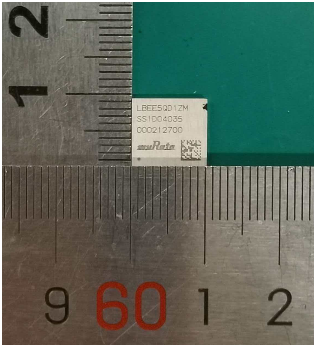
FIGURE 1 WiFi AND BLUETOOTH MODULE (LBEE5QD1ZM) FRONT APPEARANCE
