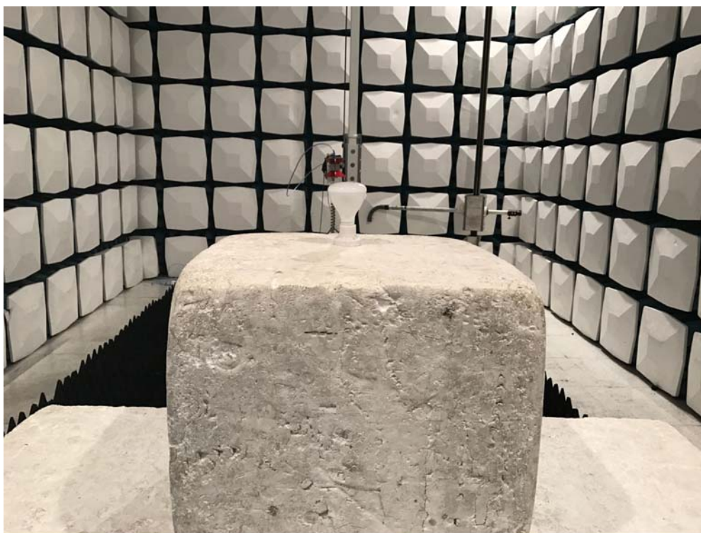
Description: Radiated Emission Test Setup for 1~18GHz
