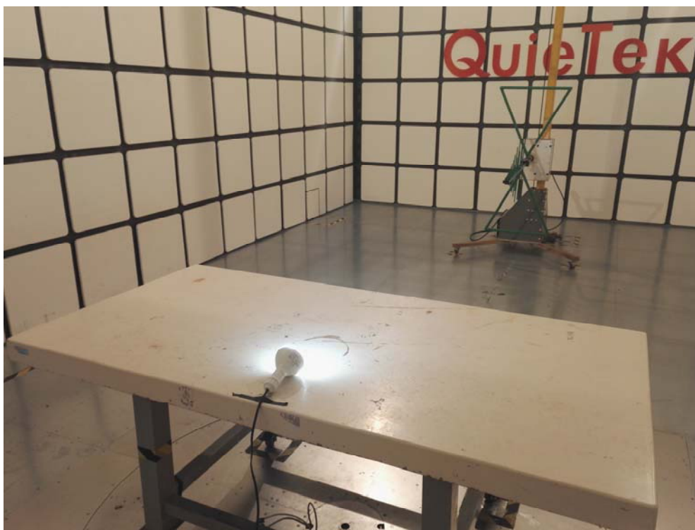
Description: Radiated Emission Test Setup for Below 1GHz
