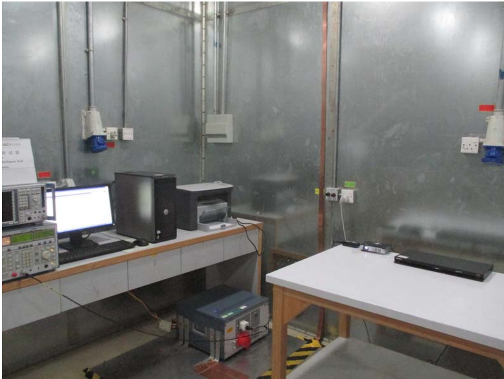
FCC RADIATED EMISSION TEST SETUP
