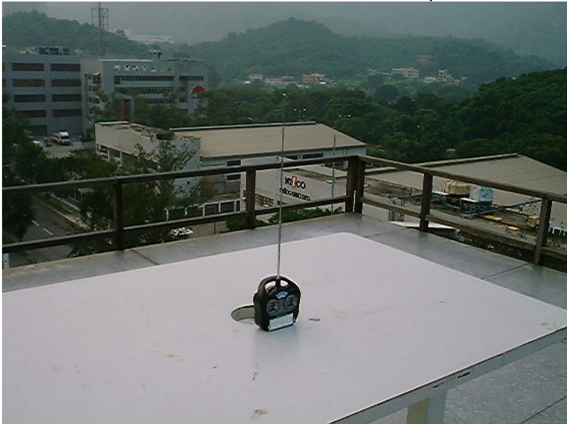
Measurement of Radiated Emission Test Set Up
