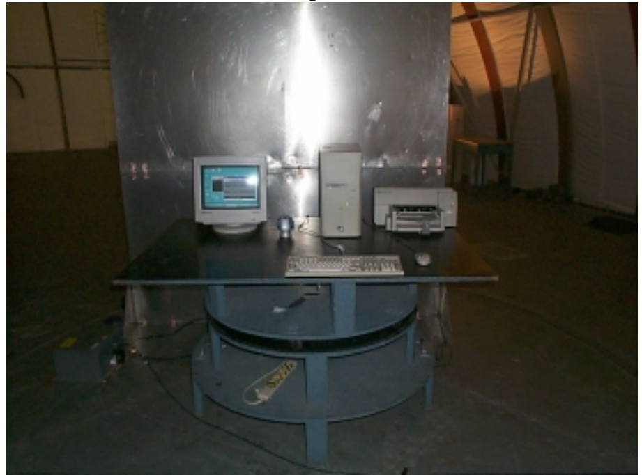
Line Conducted Emissions Test Setup, Front and Back
