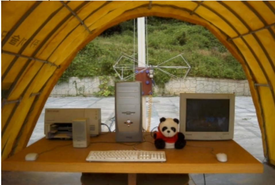
Photograph 1 : Setup for radiated Emissions
