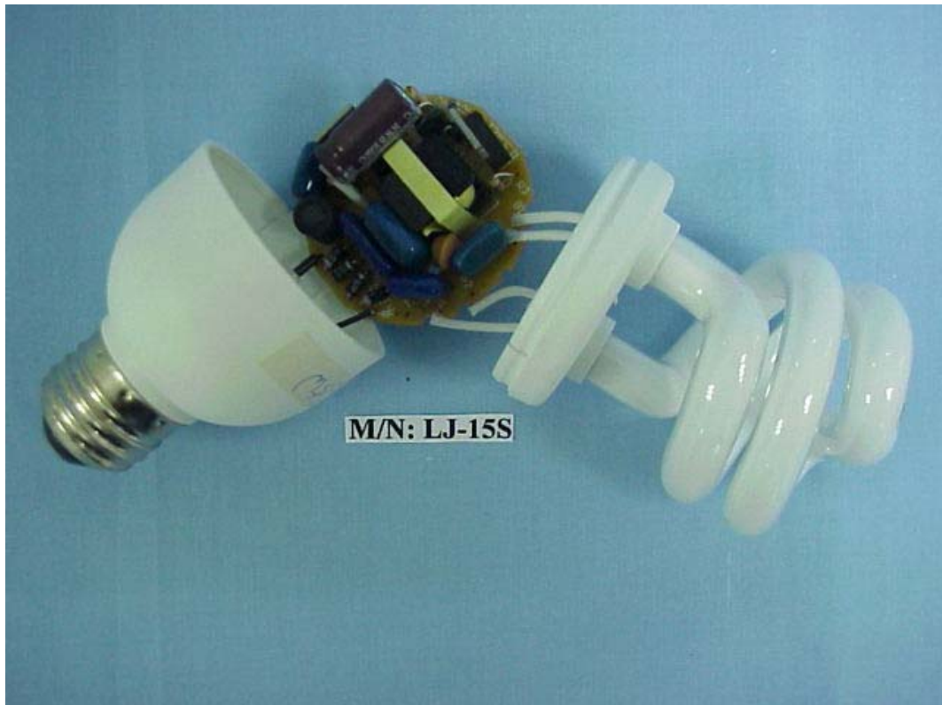
FIGURE 10 ENERGY SAVING LAMP (M/N: LJ-15S) COVER REMOVED
