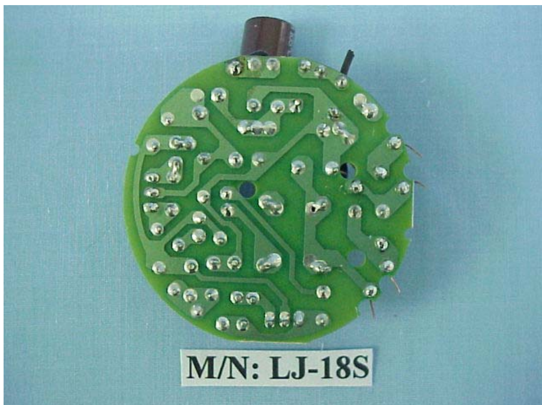
FIGURE 9 ENERGY SAVING LAMP (M/N: LJ-18S) MAIN BOARD (SOLDERED SIDE)
