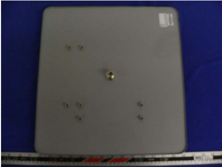
Antenna - PA58-24 REAR VIEW (5.8GHz)
