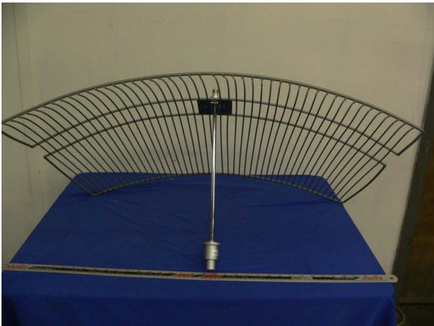
Antenna - GD53-28 FRONT VIEW (5.8GHz)
