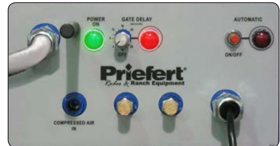
GATE DELAY "ON" & set to 4 sec.
