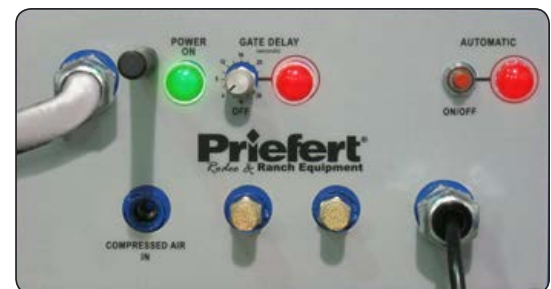
AUTOMATIC with GATE DELAY "ON" and set to 4 Seconds
