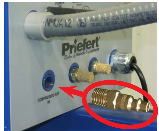
DIAGRAM 1 - Insert Fitting (Male, 1/4" NPT Quick-Connect Shown)
