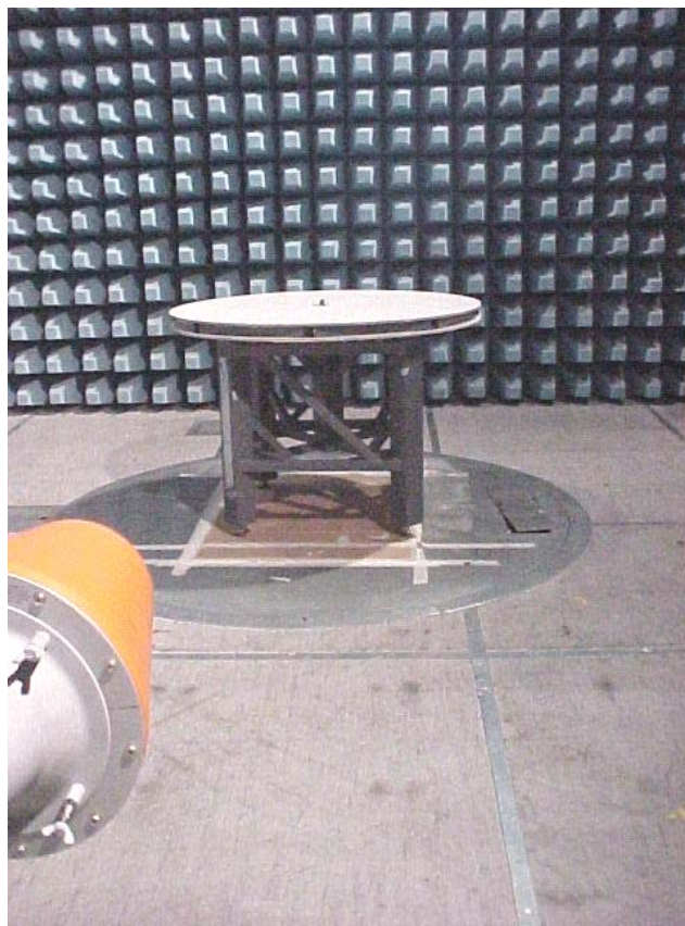
PHOTO N° 2 – SET-UP FOR EMISSION RADIATED TEST
