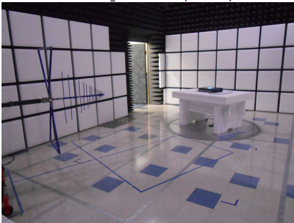
RF Radiated_ 30 – 1000 MHz #2 (rack mount)
