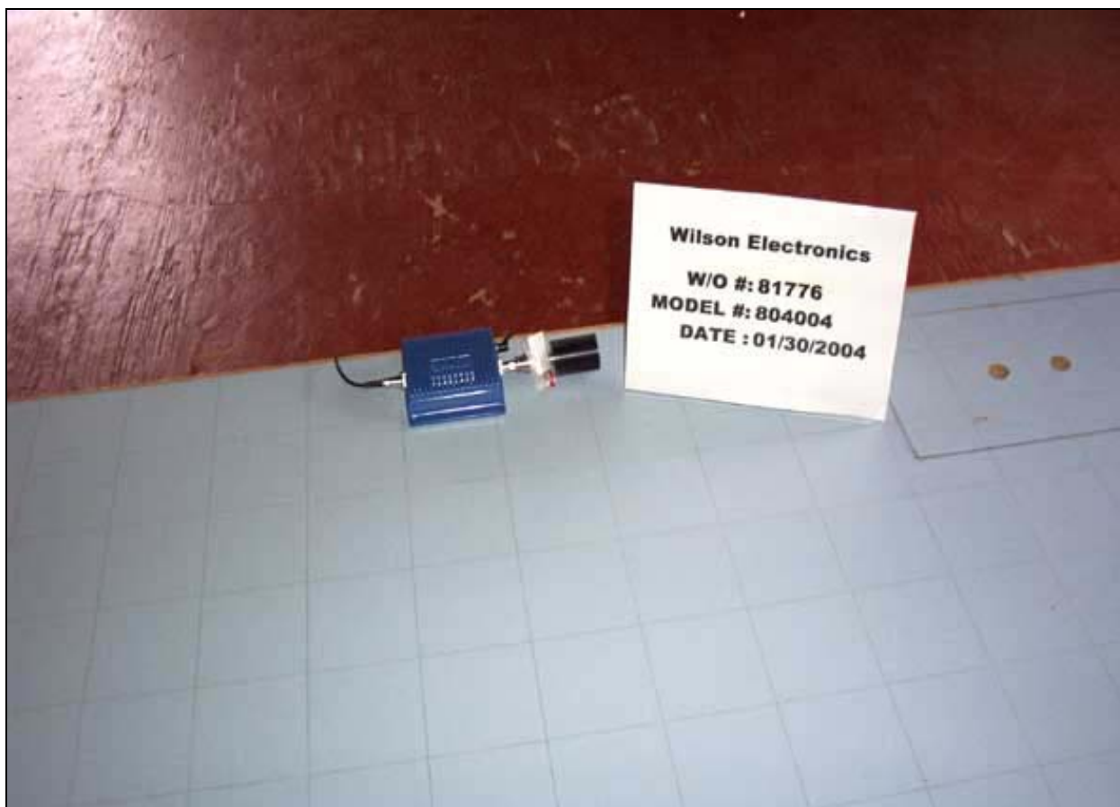
Radiated Emissions - Front View
