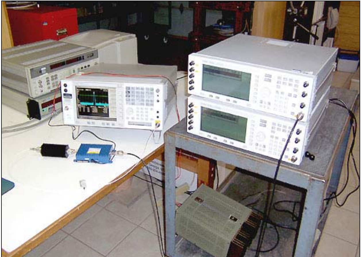
PHOTOGRAPH SHOWING DIRECT CONNECT TEST SETUP
