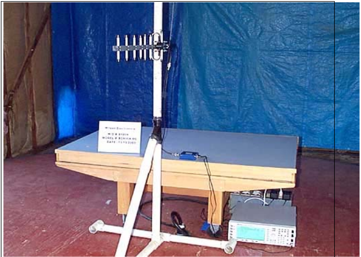
Radiated Emissions with 13 dBi Yagi Antenna
