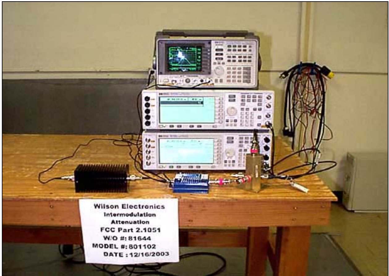
PHOTOGRAPH SHOWING INTERMODULATION ATTENUATION SETUP
