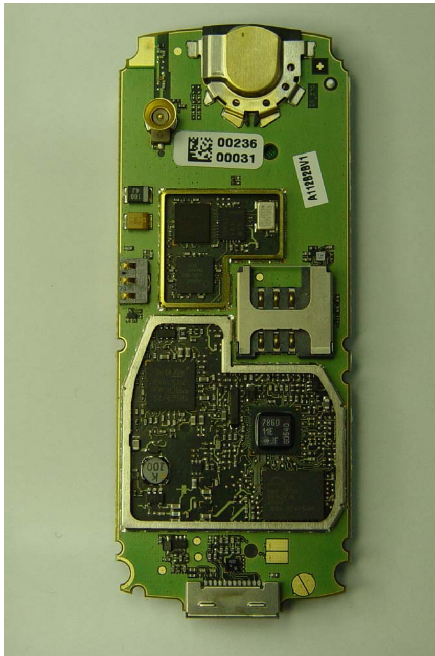
A31a PCB rear view, shielding open
