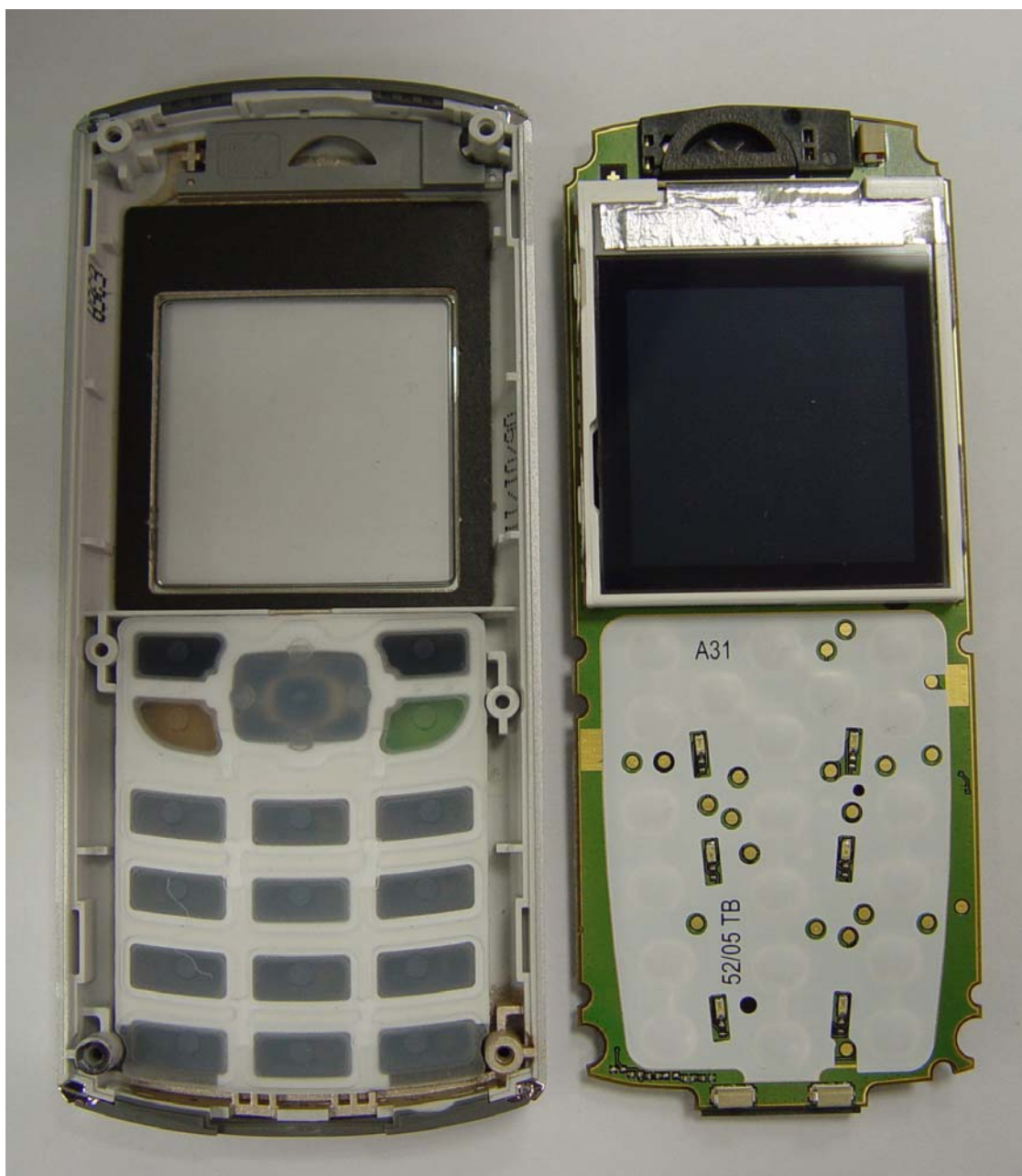
A31a disassembly step 1
