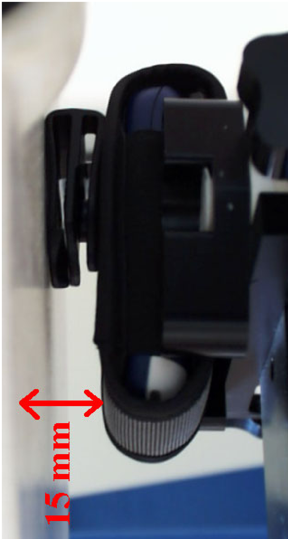
Fig. 38: Body worn configuration, Tour Case without Headset, GPRS mode (1 TX slot), Display up.
