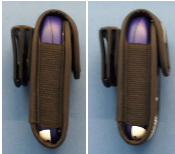
Fig. 24: Phone with used Tour Case, GPRS mode without headset and Belt Clip which dictates the closest distance to the body.
