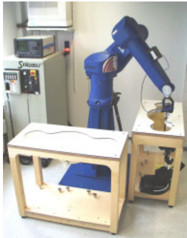
Fig. 6: The measurement set-up with two SAM phantoms containing tissue simulating liquid.
