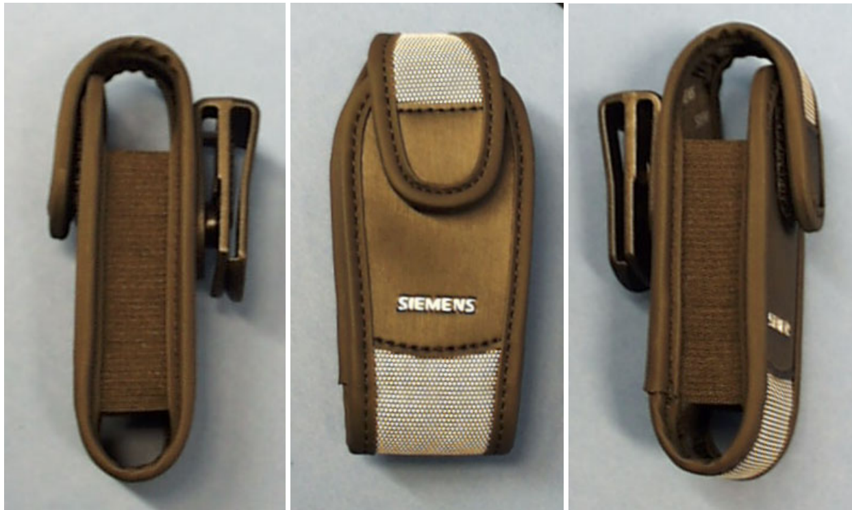
Fig. 26: Used Tour Case and Belt Clip which dictates the closest distance to the body.
