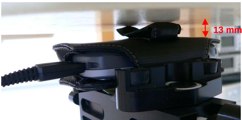
Fig. 31: Body worn configuration, GPRS mode (Class 8) with data cable, antenna towards the phantom and FCL 600 carry case.
