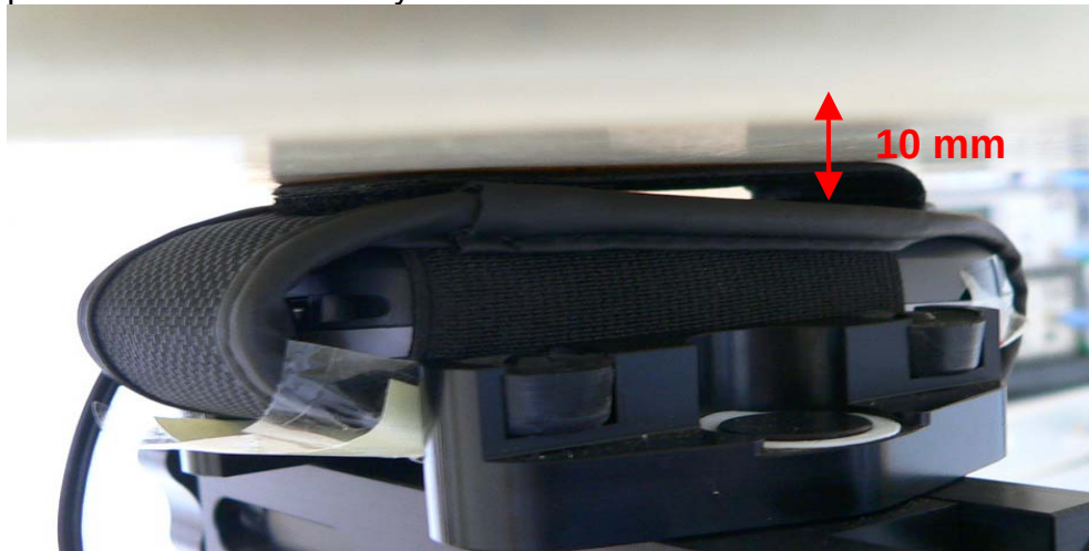
Fig. 29: Body worn configuration, GSM mode with headset, antenna towards the phantom and FCT650 carrycase.
