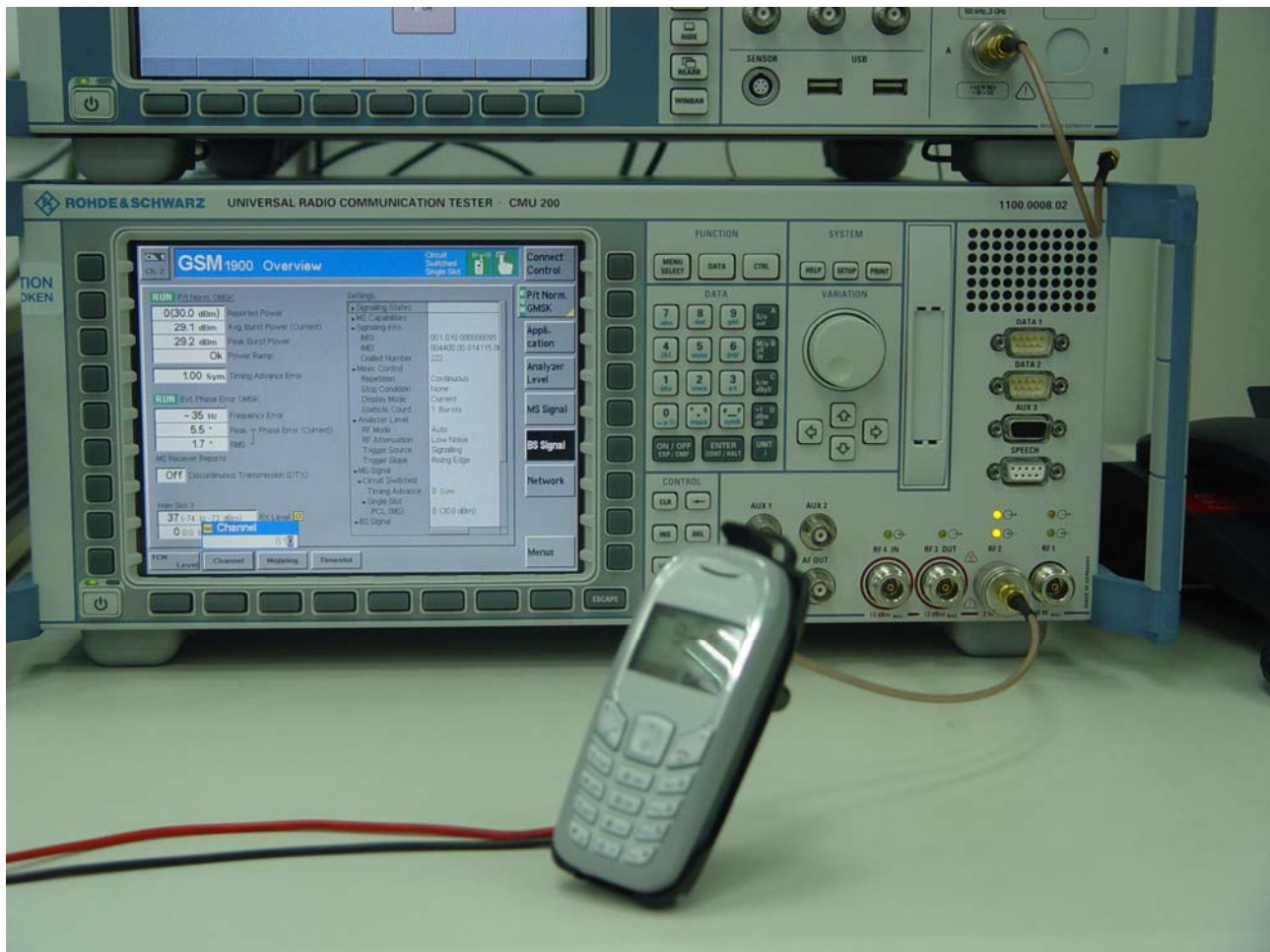
Figure 2: Set-up for conducted power measurement
