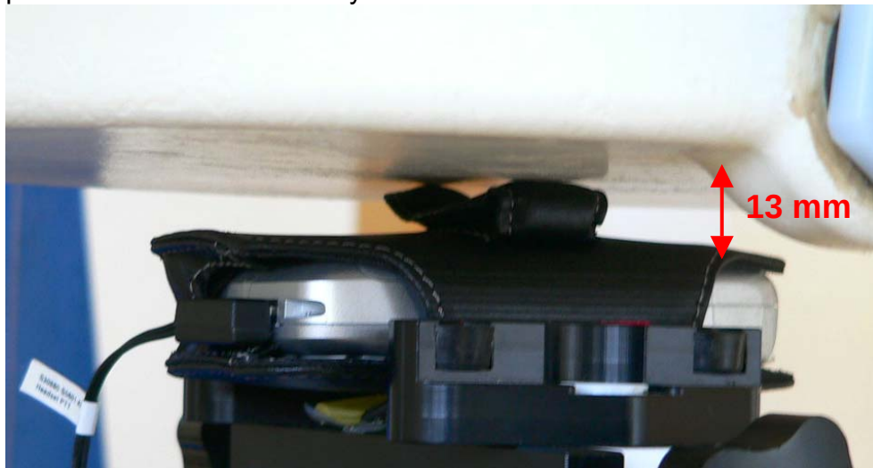
Fig. 29: Body worn configuration, GSM mode with headset, antenna towards the phantom and FCL 600 carry case.
