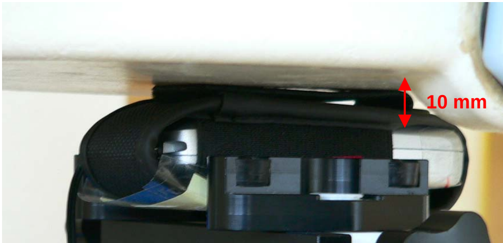
Fig. 28: Body worn configuration, GSM mode with headset, antenna towards the phantom and FCT 650 carry case.
