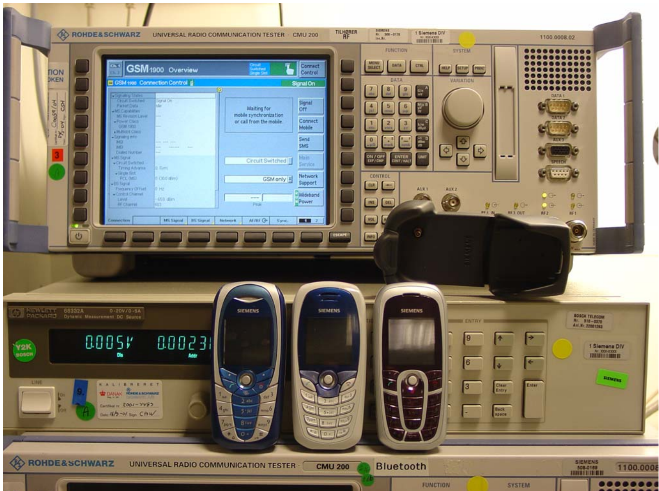
Figure 2: Set-up for conducted power measurement
