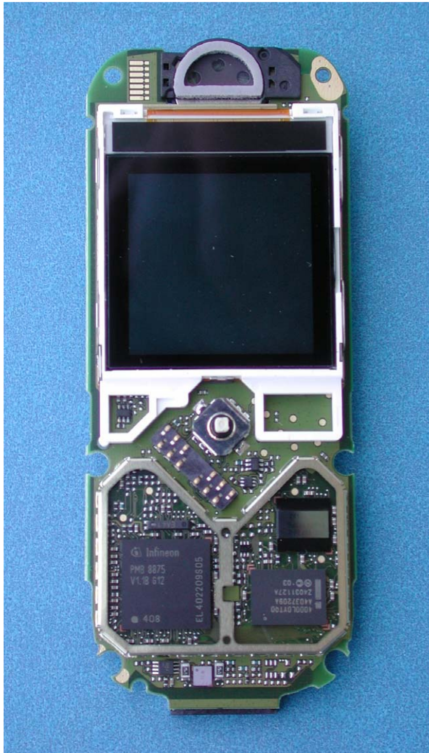
C66 PCB Front View Shields Removed
