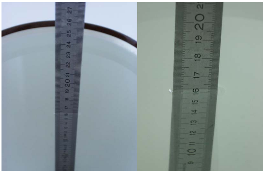
Fig. 31: Liquid depth for PCS 1900 Head and Body measurements.
