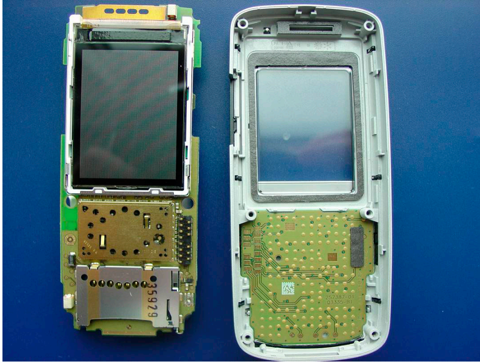
Disassemble Step 2: PCB separated from front cover
