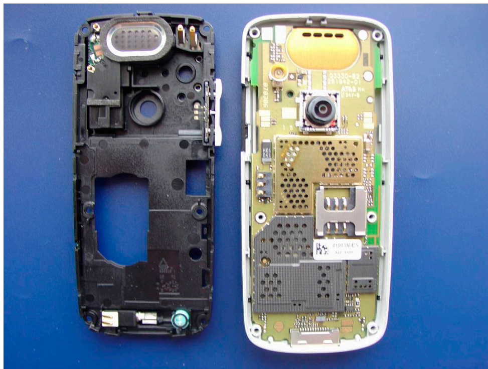
Disassemble Step 1: Lower Case opened
