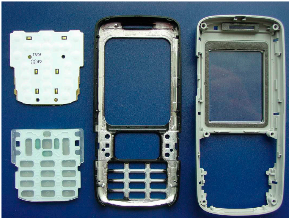
Disassemble Step 3: Front Cover disassembled
