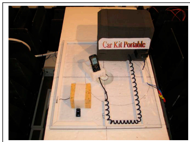
Figure 2.7 The setup for testing the Car Kit portable. The foam box contains the loudspeaker device due to the fact that the setup is also used for immunity test with respect to the European standards.
