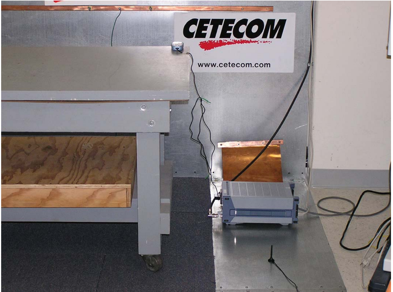
Test setup – AC Line Conducted Emissions
