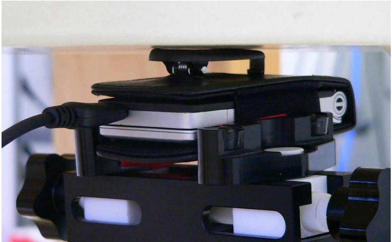
Fig. 26: Body worn configuration, GPRS (Class 10) with data cable and FCL 170 carry case, antenna towards the phantom.
