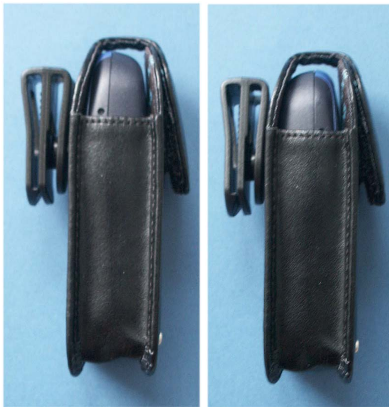
Fig. 3: Phone with leather case in the configuration: Display towards the phantom (left) and Display towards the ground (right).
