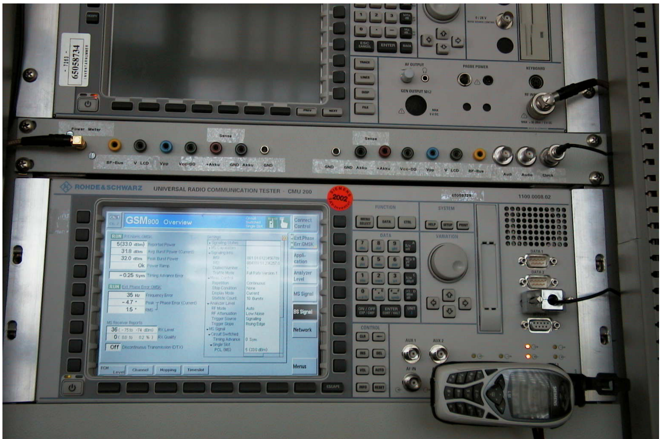
Fig. 2: Set up for conducted power measurement.
