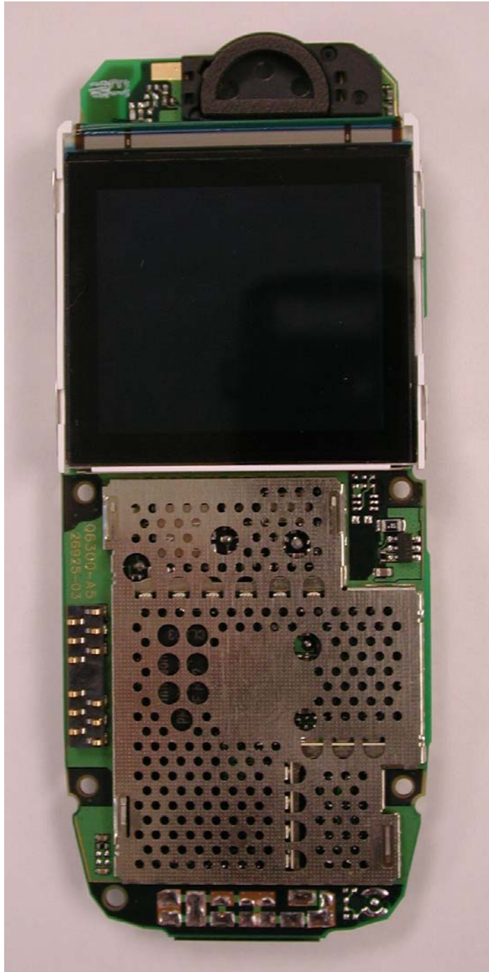
M56 Board with shielding, side 1
