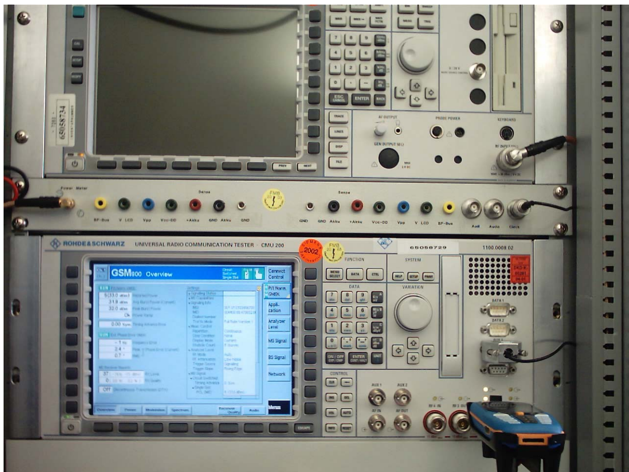
Fig. 2: Set up for conducted power measurement.
