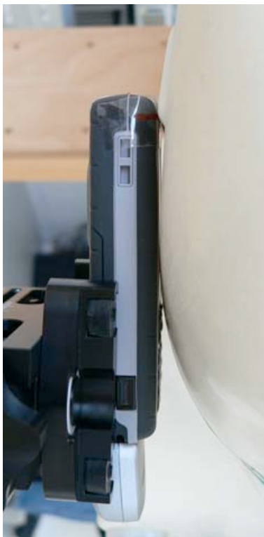
Fig. 22: Cheek position, right side with flash.
